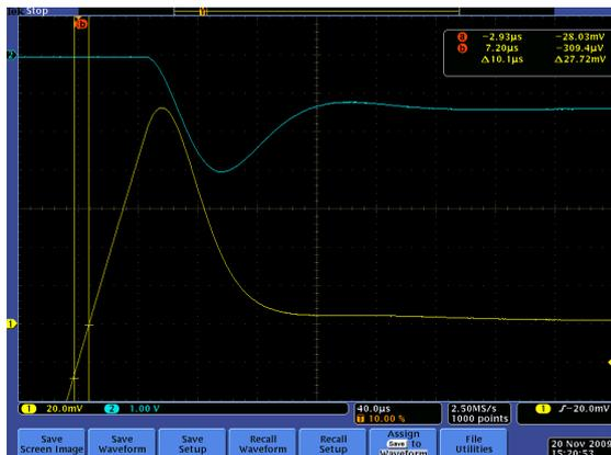
Fig.5 Reverse recovery waveforms
