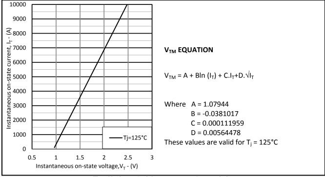
Fig.2 Maximum & minimum on-state characteristics
