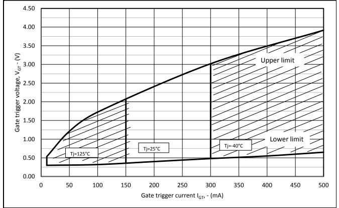
Fig.12 Gate characteristics
