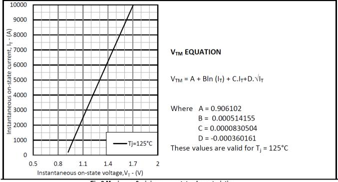
Fig.2 Maximum & minimum on-state characteristics
