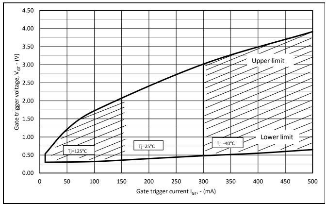
Fig.10 Gate characteristics
