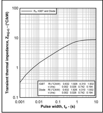
Fig. 10 Transient thermal impedance
