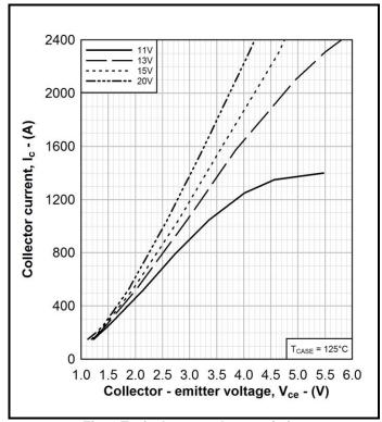
Fig. 4 Typical output characteristics
