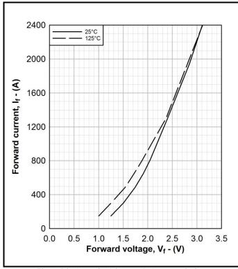
Fig. 7 Diode typical forward characteristics
