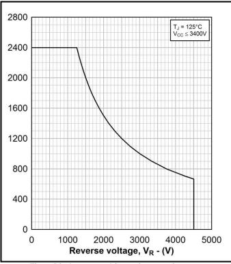
Fig. 9 Diode reverse bias safe operating area
